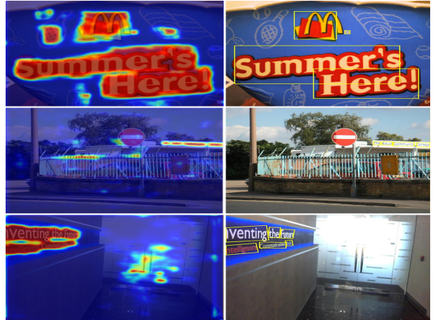
Figure 1: Illustrations of text attention mechanism in the proposed one-shot text detector. Our model automatically learns a rough text regional attention which is used to highlight text information in the convolutional features. This makes it possible to achieve accurate word-level predictions in one shot. Text can be precisely separated and accurately predicted at the word level in challenging cases.
